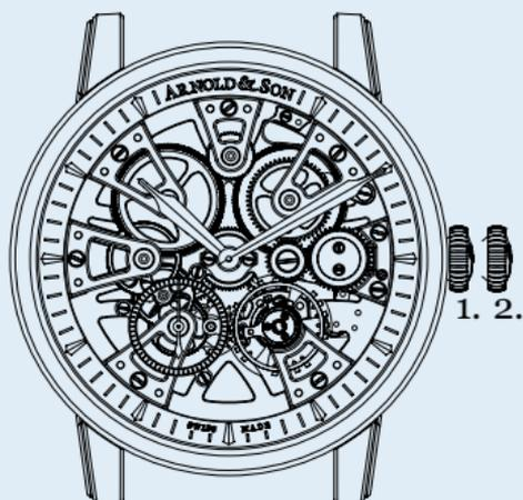
We suggest that you wind your timekeeper every 90 hours at the latest, so as to provide it with the power it requires to operate for the next 90 hours. This is how you will keep your timekeeper in a state of constant and accurate operation.
