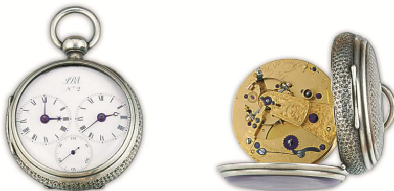
John Roger Arnold, mean and sidereal pocket chronometer with Bimetallic "Z" balance, No.2, London, 1796-1799 © Christies Bridgeman Giraudon
