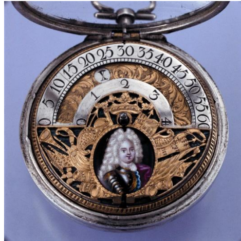
Paul Lullin, pocket watch with wandering hours indication, silver, brass and enamel, case signed AH, London, beginning of the 18 th century
