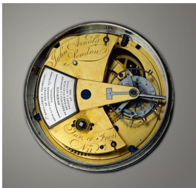
John Arnold and A.-L. Breguet, silver cased chronometer with tourbillon and spring-detent escapement, London, England, 1774 and Paris, France, 1808
