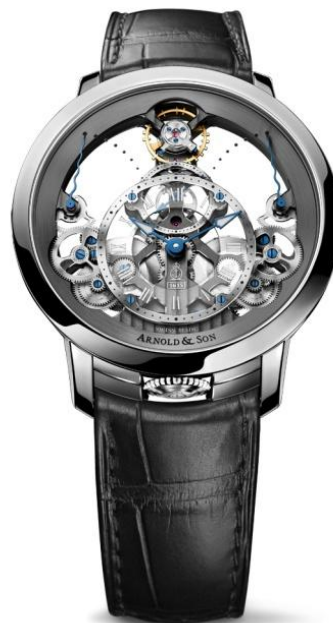
Time Pyramid Exclusive Arnold & Son skeletonised mechanical movement A&S1615, hand-wound, sapphire dial, stainless steel case, diameter 44.6 mm © Arnold & Son
